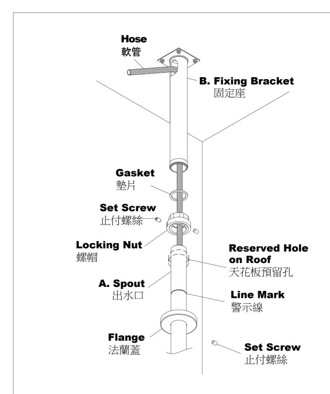
\* Disassemble Locking Nut from **Fixing Bracket** first. Insert **Spout** With Hose from the Reserved Hole on Finished Roof, and go through the Locking Nut, Gasket, and **Fixing Bracket** in sequence. Make sure Hose go out from the side hole of **Fixing Bracket**.
