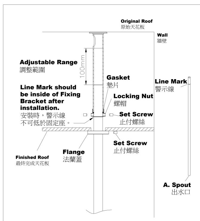
\* There are 100mm adjustable range for **Spout**, please help to make sure the Line Mark should be inside of **Fixing Bracket** after installation. After adjust the height of **Spout**, tighten the Locking Nut, fix with Set Screw on both sides, cover the Flange, and then securely fix Flange with Set Screw.
