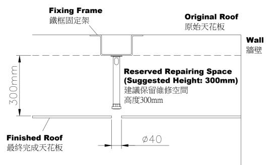
\* After install the **Fixing Bracket**, please leave the 40mm hole on the Finished Roof for next installing steps.
