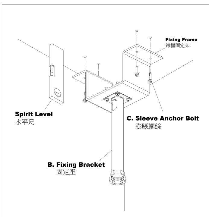
\* Select proper position for Fixing Frame Assembly, ensure the verticality with Spirit Level, use the Fixing Frame as reference to mark centers of drilling holes on the original roof, and make sure the drill holes are on the same horizontal line. Use 8mm drill-bit, drill in marked positions to 4cm depth, and then fix the Fixing Frame Assembly on the original roof with **Sleeve Anchor Bolts**.
