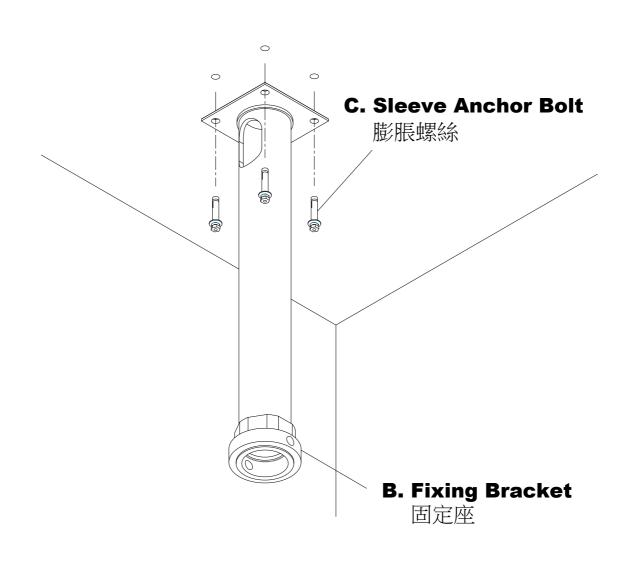
\* Use 8mm drill-bit, drill in marked positions to 4cm depth, and then fix the **Fixing Bracket** on the original roof with **Sleeve Anchor Bolts**.
