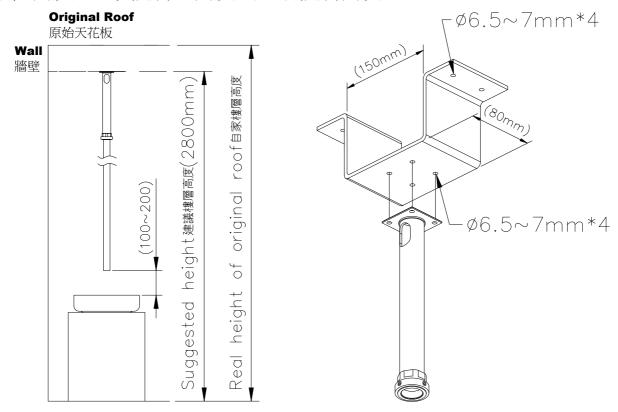
\* Please use the **Fixing Bracket** as reference to mark the drilling positions, and drill the frame with 6.5~7mm drill-bit.
