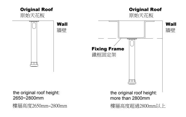
\*Available installation steps for the original roof height: 2650~2800mm 本頁適用於樓層高度為2650~2800mm
