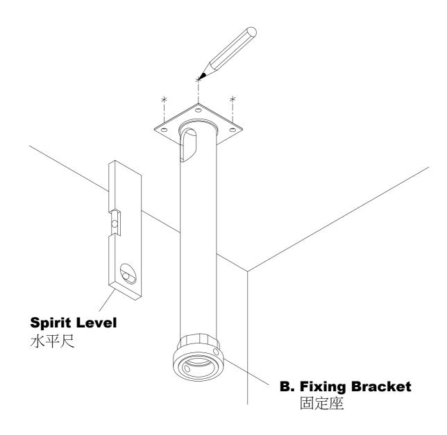
\* Select proper position for product, ensure the verticality with Spirit Level, mark centers of drilling holes on the original roof with the **Fixing Bracket**, and make sure the drill holes are on the same horizontal line.
