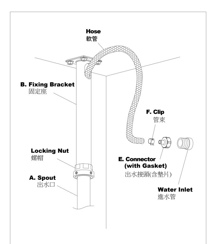
\* After install the **Spout**, screw the **Connector** to water inlet with **Gasket**, and then fix the Hose to **Connector** with **Clip**.
