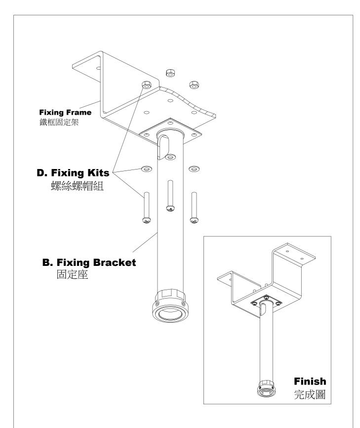
\* Fix the **Fixing Bracket** on the Frame tightly with **Fixing Kits** before installing the frame on the original roof.
