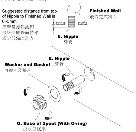
\* Apply the pipe compound or thread sealant tape and then screw it to the Valve Body. Suggested distance from top of Nipple to Finished Wall is 0~5mm, and Nipple could be cut if necessary. Screw the Base of Spout (With O-ring) with Gasket and Washer clockwise to Nipple till against Finished Wall. Please notice the Gasket has to be placed between base and wall.
