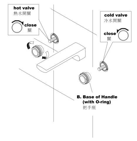
\* Turn the spindles of valves to closed position, screw the **Base of Handle** to the shanks of **hot and cold valves** till against finished wall.
