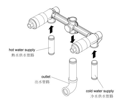
\* Install hot and cold water supply pipes and outlet.
