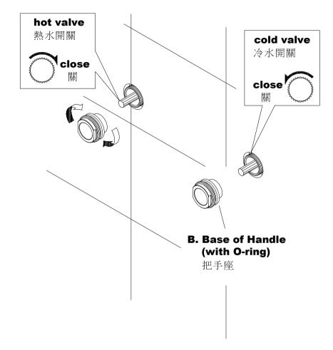
\* STurn the spindles of valves to closed position, screw the **Base of Handle** to the shanks of **hot and cold valves** till against finished wall.
