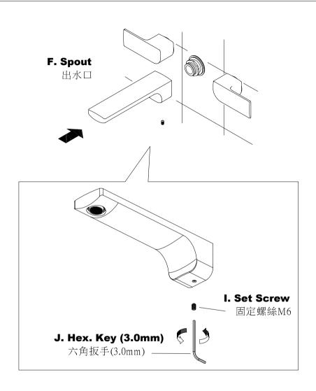
\* Position **Spout** onto **Base of Spout**, and then fix with provided **Set Screw** and **Hex Key**.
