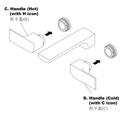
\* Confirm hot and cold valves have been turned to closed position before install the **Handles**. Press hot and cold **Handles** onto valve spindles until hear the click sound as the figure shows.
